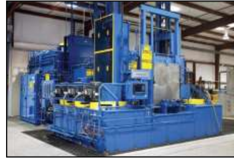
Fig 6: Integral quench atmosphere furnace equipped with 41 m3 IQ water tank built by AFC-Holcroft and installed at Euclid heat treating Co [10].
