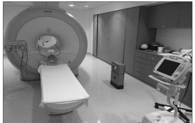
Fig 3: A front-facing patient table, capable of being repositioned within the magnet's bore, is a feature of the clinical MRI system.
