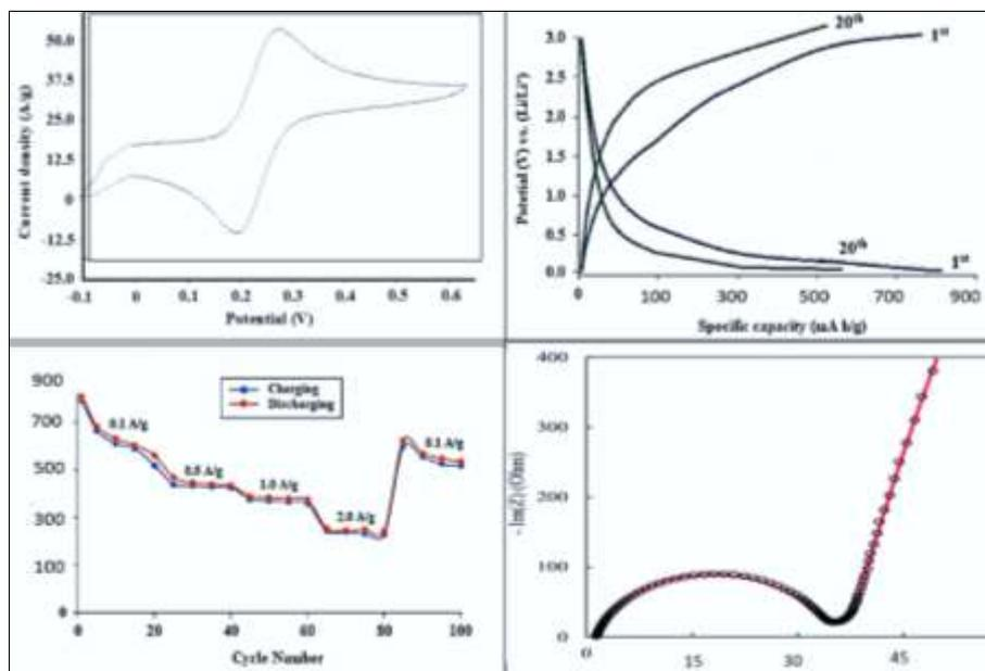
**Fig 6:** Electrochemical performance of Ni-BCA/CF composite anode material against lithium cathode in 1M  $\text{LiPF}_6$  electrolyte.
