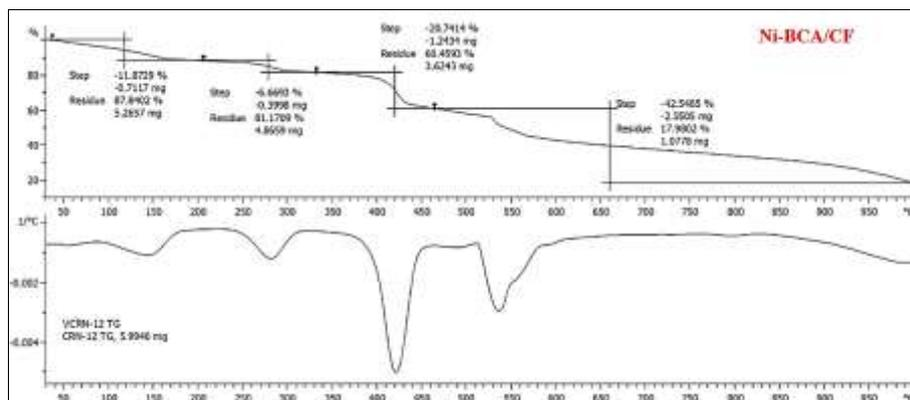
**Fig 4:** TGA studies to assess the thermal stability of the Ni-BCA/CF composite
