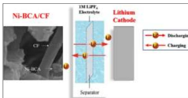
**Fig 1:** Schematic illustration for Ni- BCA /CF hybrid composite Anode material and lithium foil as a cathode in 1M LiPF<sub>6</sub> electrolyte.
