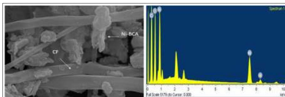
**Fig 5:** SEM and EDS to assess the morphology of Ni-BCA/CF composite
