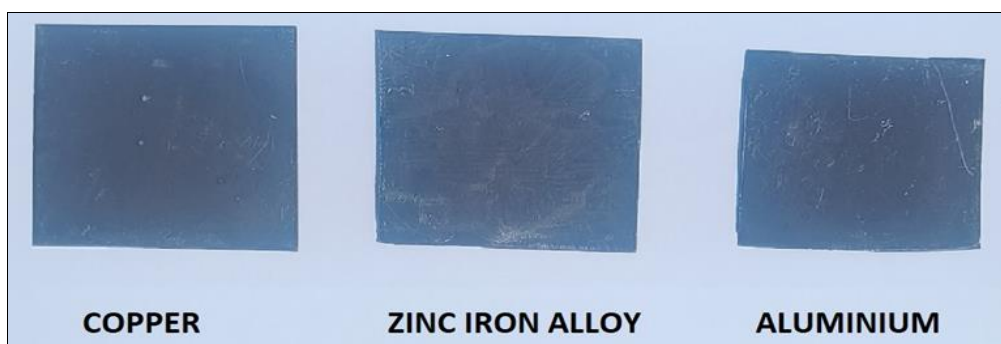
Fig 2: Nano carbon and copper oxide coated solar absorbers
