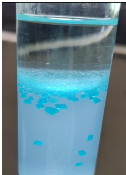
Fig 2: Growth of copper tartrate crystal
