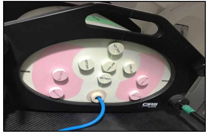
Fig 1: CIRS Thorax phantom with ionization chamber
